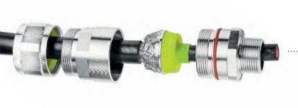
The rubber pad is mounted internally to the cable press backnut and has no chance of getting out freely, avoiding accidental loss. Also to avoid the risk of loss, the reinforcement ring is fixed to the intermediate.
